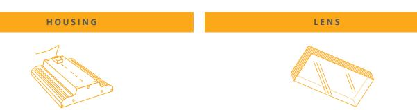
Durable outer shell that protects and positions the light source; sound mechanical engineering prevents corrosion and humidity from degrading electrical components.
